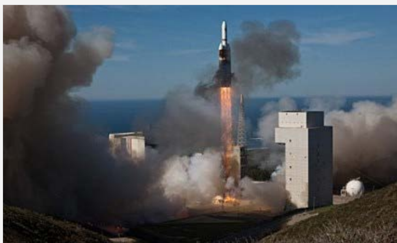
A Delta IV Heavy lifts off from Vandenberg AFB in January, 2011, the insulation on the outside of the rocket blackened and still burning as the launch vehicle clears the pad. (Photo: United Launch Alliance, LLC)
