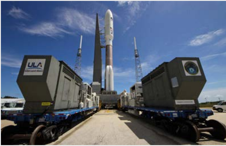
The Navy's second Mobile User Objective System (MUOS) communications satellite was launched in July 2013 aboard the most powerful and fastest version of the Atlas V, equipped with five solid rocket boosters. (Photo: United Launch Alliance LLC)
