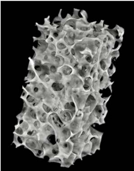
Computerized tomography (CT) scan of the implant structure. (Image: Neil Ives)
