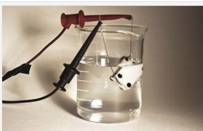
Hydrogen and oxygen being generated through electrolysis of water with a polymer electrolyte membrane. (Photo: Elisa Haber)
