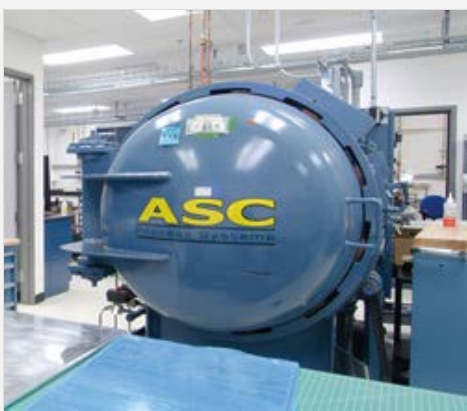
High-performance autoclave in the Advanced Composites Laboratory used for the fabrication of advanced component material test articles. (Photo: Eric Hamburg)
