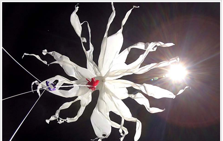
A weather balloon carrying a test version of Aerospace's Mars lander bursts at 80,000 feet over the Nevada desert. (Photo: The Aerospace Corporation)
