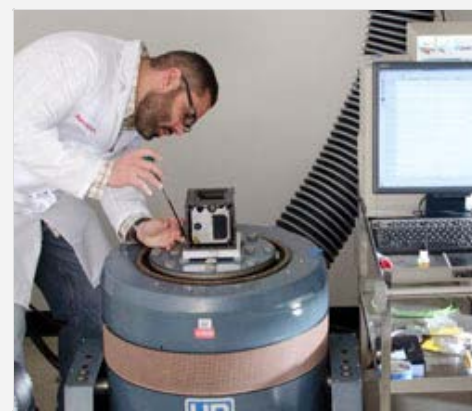
Manuel Acosta setting up a CubeSat for launch vibration load testing in the Fluid Mechanics Lab. (Photo: Eric Hamburg)
