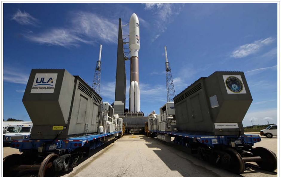
An Atlas V rocket carrying the Navy's MUOS-2 satellite is transported from the Vertical Integration Facility to the launch pad at Space Launch Complex 41 at Cape Canaveral. (Photo: United Launch Alliance, LLC)
