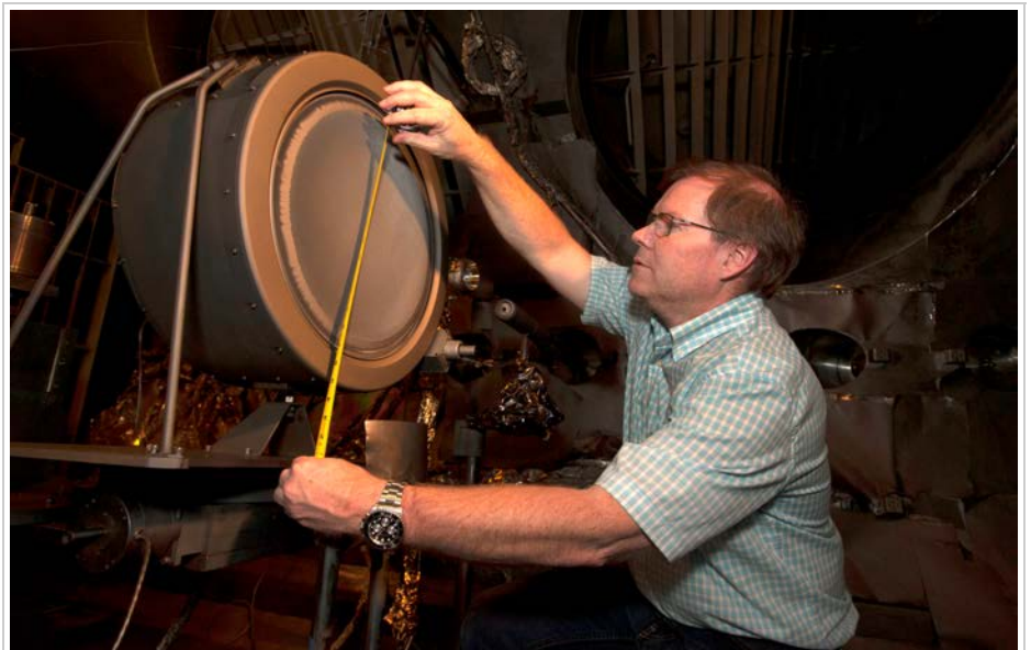
Mark Crofton, senior scientist, Propulsion Science Department, measures movements made by the NASA Evolutionary Xenon Thruster (NEXT) during testing. (Photo: Heather Golden)
