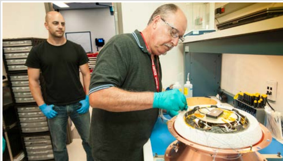
Geoff Maul, of the Microsatellite Systems Department, looks on while Asuncion (Jose) Perez of Boeing prepares the heat shield of the next Reentry Breakup Recorder for sealing. The REBR was sent to NASA on Monday, July 14, and is scheduled to launch in October on the Orb-3 resupply mission to the International Space Station. (Photo: Eric Hamburg)
