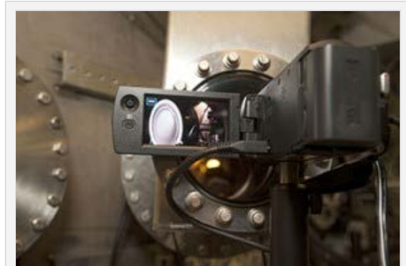
A video camera records the NEXT as it operates within a vacuum chamber at Aerospace. (Photo: Heather Golden)
