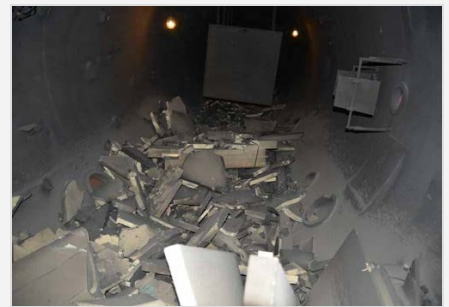
DebrisLV debris field 50 ft downrange.
