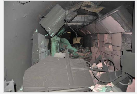
...and after. The cables hanging from the ceiling are where DebrisSat had been hanging.
