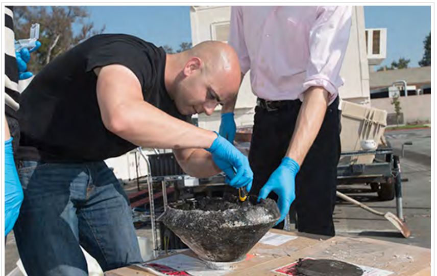
Geoff Maul removes the burnt electronics payload from the REBR-W on Monday, March 30. (Photo: Eric Hamburg)
