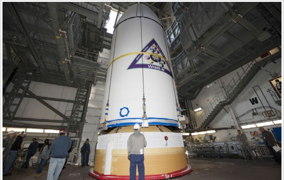
The WGS-8 satellite, encapsulated in its payload fairing, is attached atop a Delta IV rocket at Cape Canaveral Air Force Station. (Photo: United Launch Alliance, LLC)
