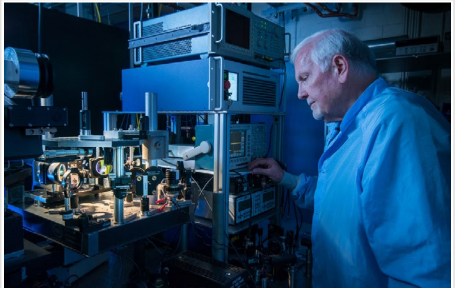
Bill Hansen, who has since retired, works with equipment used to detect defects as 3-D printed products are being made. (Photo: Eric Hamburg)
