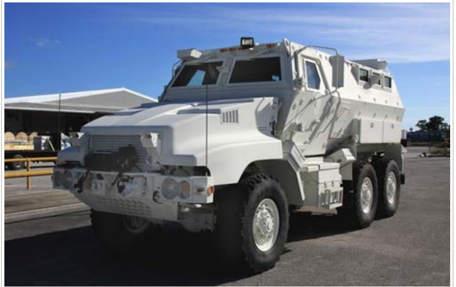
Space Launch System astronauts will board this Mine-Resistant Ambush-Protection (MRAP) vehicle or an identical MRAP, which will carry them away from Launch Complex 39 in the event of an emergency. (Photo: NASA/Jim Grossman)
