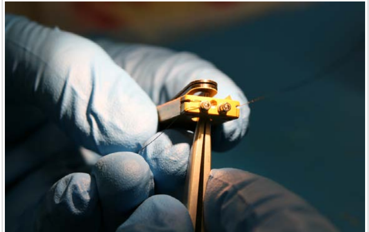
A shape-memory actuator will release solar arrays on the upcoming Optical Communications and Sensor Demonstration mission. (Photo: Aerospace)
