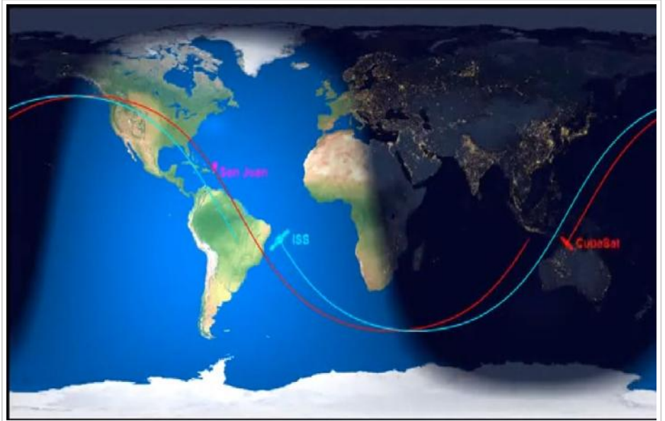
In this fictional demonstration, the Rollercoaster CONOPS is used to survey damage to San Juan after a hurricane strikes Puerto Rico. The Rollercoaster CubeSat achieves a flyby over San Juan in ~27 hours, whereas the ISS (from which it's deployed) would not have such a viewing opportunity for tens of days.
