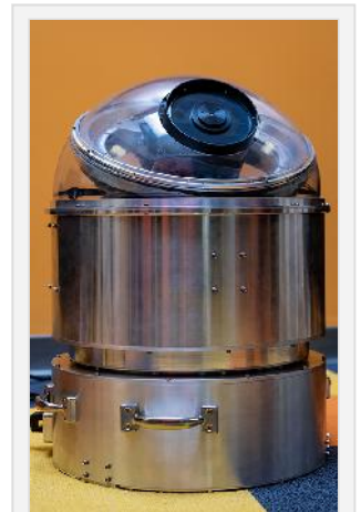
The Monocle prototype features a dome enclosure that protects the optics from outside elements.
