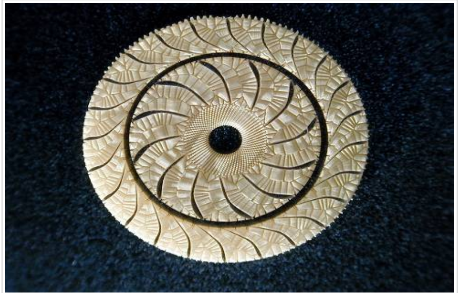
A counter-rotating turbine, fabricated in photostructurable glass ceramic material using a novel Aerospace laser machining technique.
