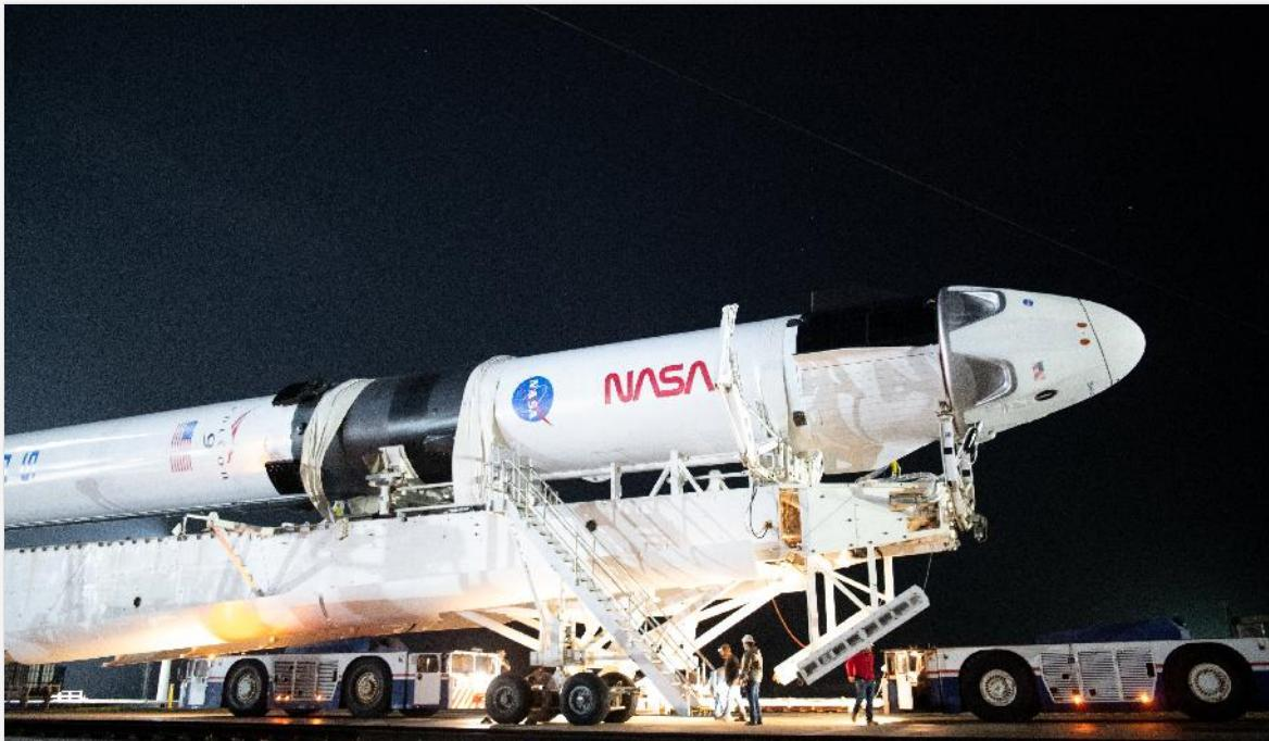
A SpaceX Falcon 9 rocket with the company's Crew Dragon spacecraft onboard is seen on the launch pad at Launch Complex 39A before being raised into a vertical position, Monday, Nov. 9, 2020, at NASA's Kennedy Space Center in Florida. Photo Credit: (NASA/Joel Kowsky)
