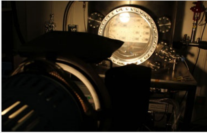
Solar cells undergo testing inside a thermal-vacuum chamber while a light shines through. Chamber conditions simulate a space-like vacuum where the solar cells are cooled to a temperature of minus 60 degrees Celsius. (Photo: Justin Lee)
