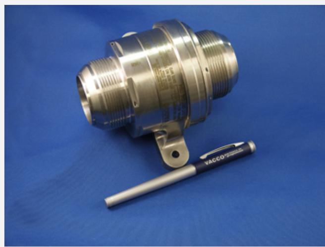
A Delta IV cryogenic valve, one of many pieces of hardware that Aerospace helps review in preparation for launch. (Photo: VACCO Industries)
