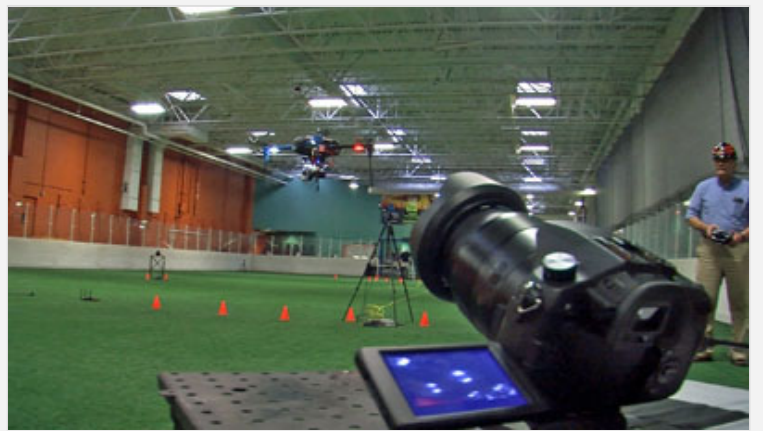
One of the cameras collects footage of the drone and sends it to the on-site computer to be converted into a real-time 3-D track. (Photo: Lester Chung)
