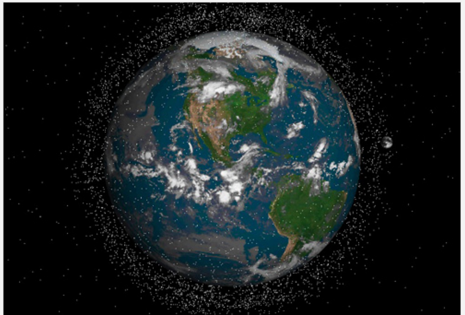
A graphic representation of the debris orbiting Earth, created with Aerospace's Satellite Orbit Analysis Program. (Graphic: John Coggi)
