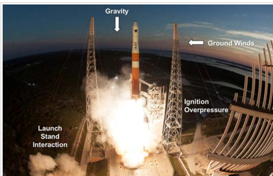
At each point during the launch and ascent, a variety of loads are affecting the vehicle. (Photo: United Launch Alliance, LLC)
