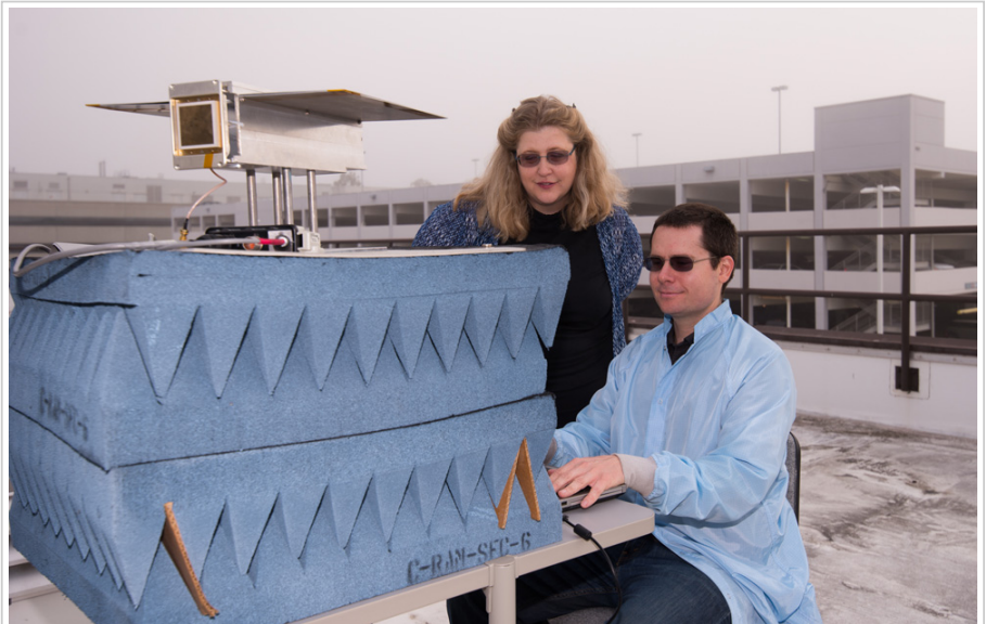
Dr. Rebecca Bishop and Steve Biel test the sensor that Aerospace will contribute to the SPORT CubeSat. (Photo: Eric Hamburg)
