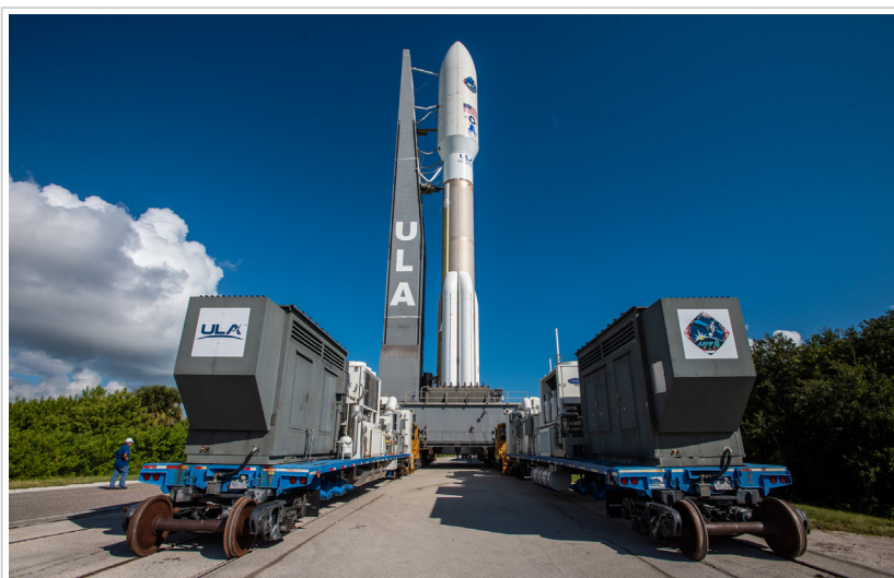
An Atlas V rocket with the AEHF-4 spacecraft rolls from the Vertical Integration Facility to the launch pad at Cape Canaveral Air Force Station. (Photo: United Launch Alliance, LLC)
