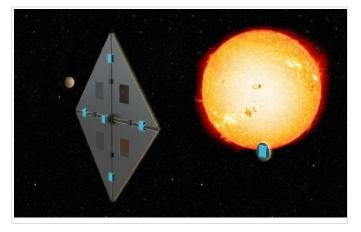
Solar sails harness the radiation pressure exerted by light on a reflective material to provide thrust to spacecraft. With few moving parts and the propellant offboard, solar sails provide cost-effective operations and long operating lifetimes. The technology is proven, and was successfully demonstrated by Japan's IKAROS mission's fly-by of Venus in 2010.
