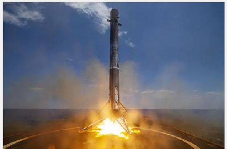
Recovery of the Falcon 9's first stage on a drone ship. (Photo Credit: SpaceX)
