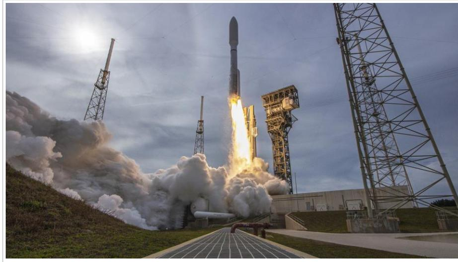
The USSF-8 mission to geosynchronous orbit (GEO) was the first and only planned use of an Atlas V 511 launch vehicle configuration. The 511 launch vehicle is a unique configuration that uses one of the short five-meter payload fairings and only one strap-on solid rocket booster along with a single engine Centaur III upper stage.
