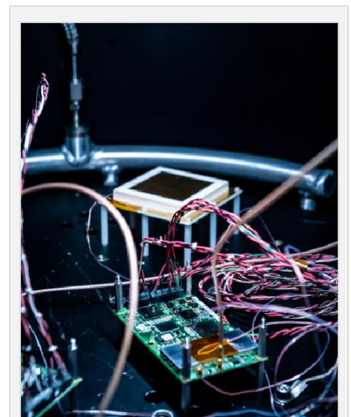
Aerospace contributed the Compact Total Electron Content Sensor (CTECS), a GPS radio occultation (RO) sensor, for the SPORT mission.
