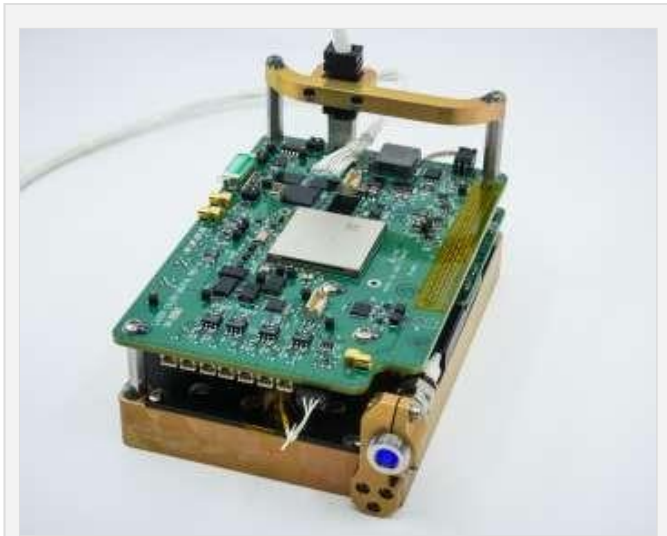
Lasercomm, Slingshot's next-gen laser communications downlink.
