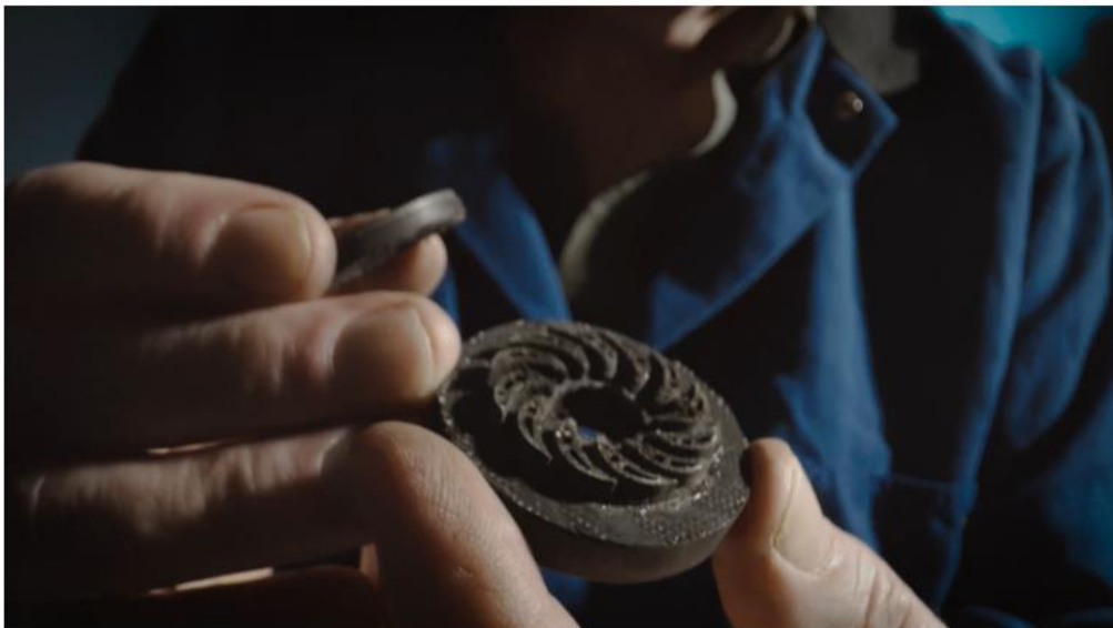
The deflector plate from the Deorbit Motor forces gases through various vanes circling the plate, causing the entire satellite to rotate.
